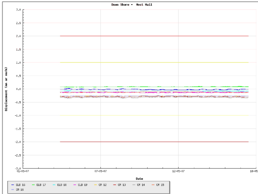
Figure 3: Time-displacement plot of devices installed in the western most tunnel.
